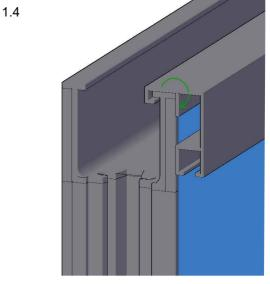
Then the picture rail rotates and alignes itself to the surface of Mila-Wall.
