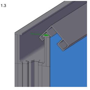
Move the picture rail forward until the slot grabs into lip.
